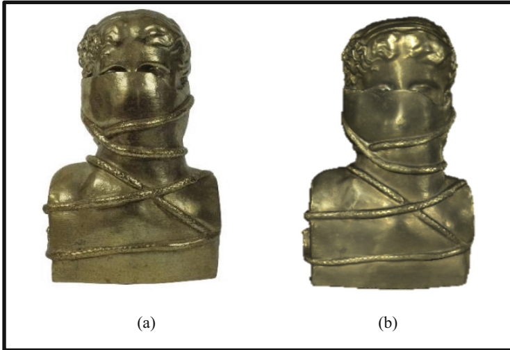
Fig. 2. (a) Photograph of an artifact (b) 3D representation produced by employing a structured light scanner.
