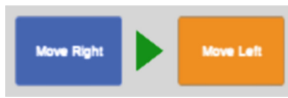
Fig. 8. A transition between two states of an FSM represented by a green triangle. (Color figure online)
