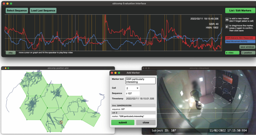
Fig. 2. The Evaluation Viewer : timeline with event markers and plots of GSR and head movement, position tracking on ground floor plan, video composed of camera recordings, editor for manual markers
