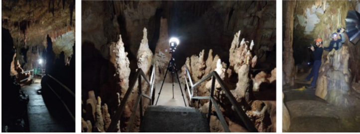
Fig. 5. 3D scanning process inside the cave
