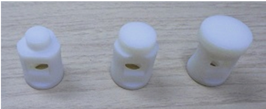
Fig. 5. Contact heads with different radii (from left to right: \phi 10 , \phi 15 , and \phi 20 ). The \phi 10 mm contact head was close to the area of the biceps brachii tendon.
