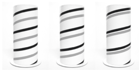
Line afterimage from 150 rpm to 600 rpm (left to right)
