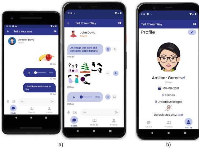
Fig. 4. Illustrative screens of the first functional prototype running on Android and depicting: (a) both sides of a conversation between John David and Jennifer Days with different messages conversions (image-to-text; audio-to-image; and text-to-audio); and (b) Amilcar's profile screen showing his preferred modality and disabilities.
