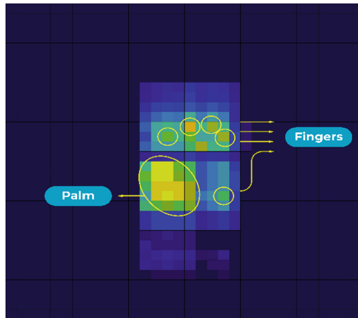
Fig. 3. The pressure distribution when one hand is pressed on the mat.
