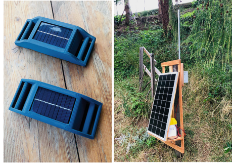
Fig. 1. Two components of the ViehFinder setup, solar powered ViehFinder node (left) and LoRaWAN antenna (right).
