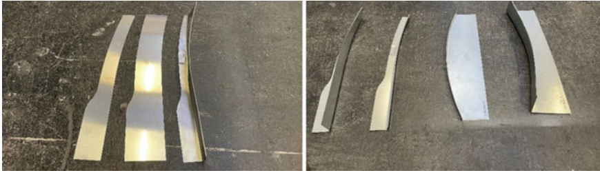
Fig. 13 Bending results 3D-swivel-bending
