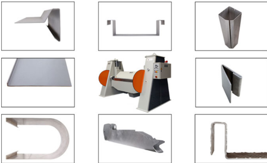
Fig. 3 Geometric manufacturing range of CNC swivel-bending machines (center image) according to [2]
