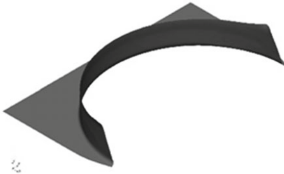
Fig. 8 Semi-circular concave cross-section geometry
