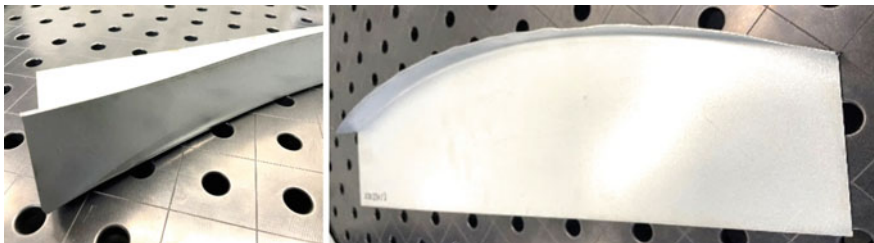
Fig. 9 Wrinkling as a case of failure—concave (left), convex (right)
