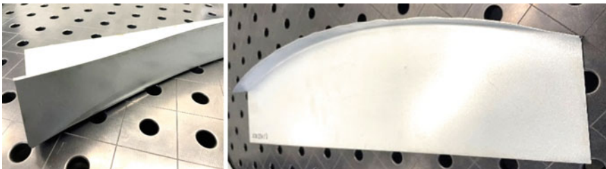
Fig. 9 Wrinkling as a case of failure—concave (left), convex (right)
