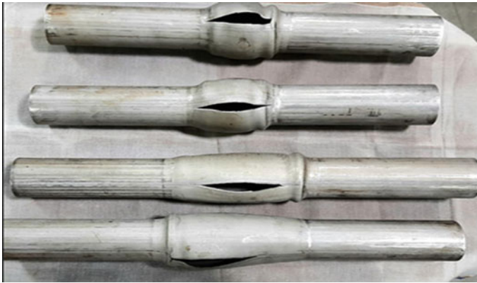
Fig. 4 Fracture location in deformed tubes
