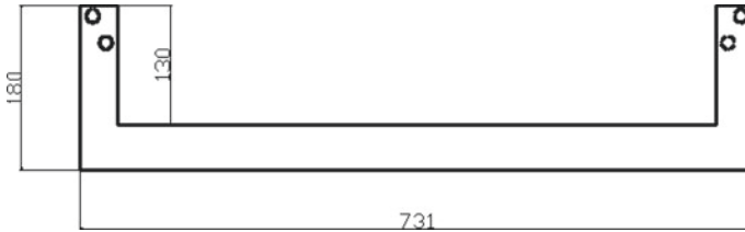
Fig. 1 The size of specimen for electrically-assisted draw-bending test (unit: mm)
