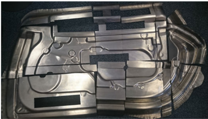
Fig. 11 Door inner sections cut for thickness evaluation
