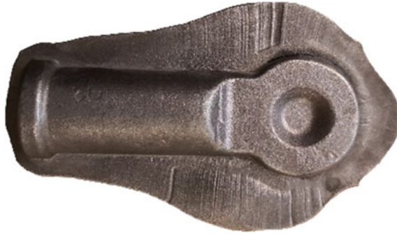
Fig. 2 Conventional forging of Tongue. 25% of the material is wasted in the flash form
