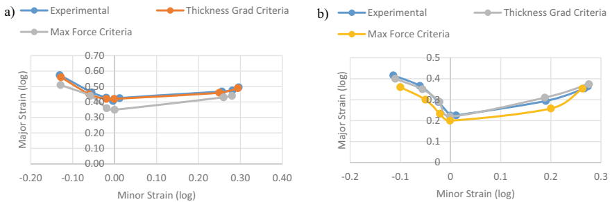
Fig. 10 Comparison of model predicted FLD with punch load and 0.92 thickness gradient criterion with experimental FLD for a AA5052, b AA5083
