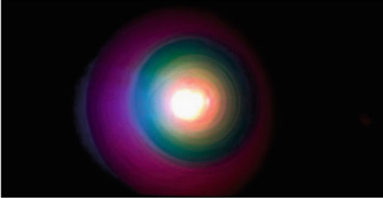
Fig. 11.1 Rings of anti-Stokes conical emission surrounding a white supercontinuum center. Image shows how colorful rings of red, orange, yellow green, blue, and violet spread out angularly from a central white light supercontinuum signal
