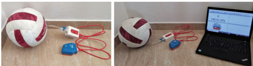
Fig. 3 Left: Apparatus for measurement of pressure, in the process of apparatus design. Right: Air pressure in the ball measurement in Coach 7
