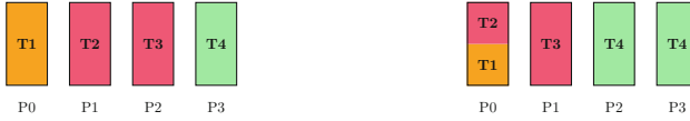
Fig. 2. Left: 4 equal-sized tasks on 4 cores, each with allocation a_j = 1 . Right: 4 tasks with exponentially increasing workloads on 4 cores with allocations 0.5, 0.5, 1, 2, resp.
