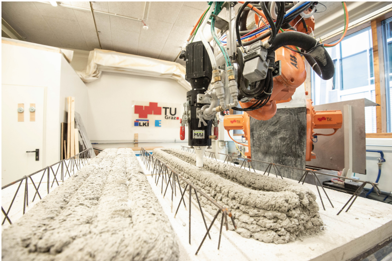
Fig. 5. Prototype of an element slab with printed AFC – 150 to 280 kg/m 3
