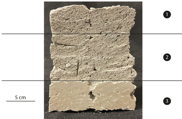
Fig. 3. Printed specimen of adaptive foam concrete (AFC) with varying density conversion during the printing process. (1) 150 kg/m 3 ; (2) 280 kg/m 3 ; (3) 1070 kg/m 3
