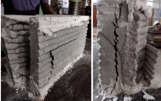
Fig. 4. Crack propagation in printed wall element
