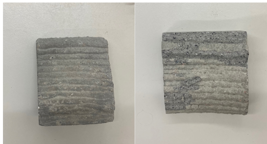
Fig. 2. Samples at 0 cycles (left) and 300 cycles (right) of freeze-thaw. During thawing, samples were immersed in water in the same way as shown in picture with the surface having maximum area facing downward.
