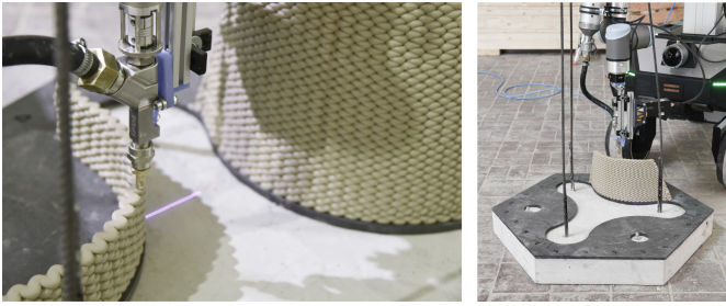
Fig. 5. Clay extrusion of segment 1 (right) and 2 (left)
