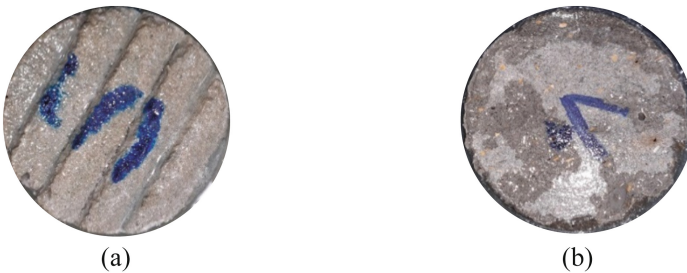
Fig. 2. Salt scaling damages observed on (a) printed and (b) mould cast samples.
