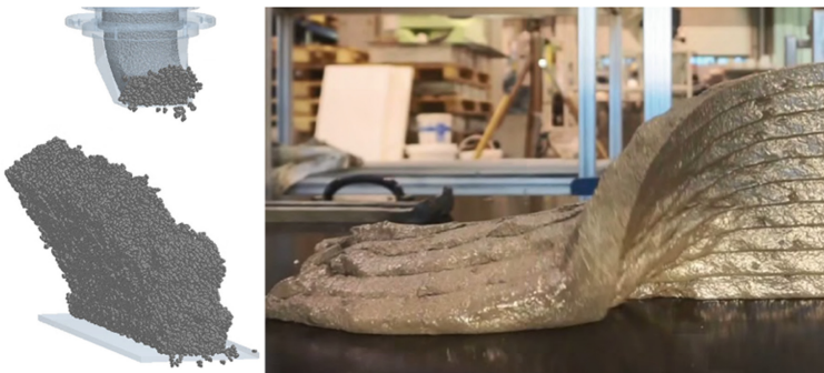
Fig. 4. DEM simulation (left) and real application (right) of a multi-layer concrete print with insufficient material stability leading to a collapse of the layers, shown from different angles.
