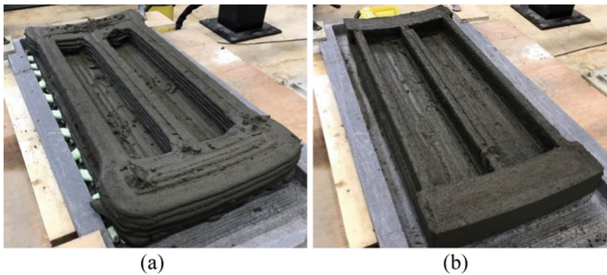
Fig. 3. A) The printed part (near-net-shape) and b) the part post-milling (net-shape).
