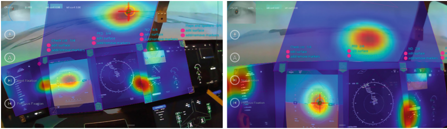
Fig. 6. Attention distributions among different displays on the flight deck shown as heatmap between PF (left) and PM (right)
