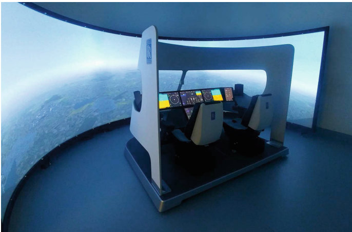
Fig. 1. Future Systems Simulator (FSS), located at Cranfield University. The flight deck consists of touchscreen monitors and the cockpit is modular and fully reconfigurable; the shroud can also be taken away to accommodate simulation of drone flight or air traffic management.
