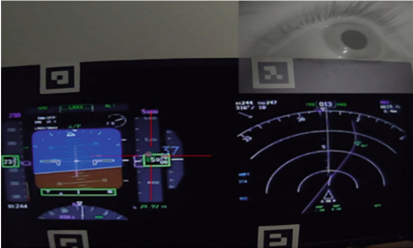
Fig. 1. Pilot's fixation at the altitude indicator (red-cross) and pupil dilation (right-hand side) on augmented design of PFD recorded by Pupil Eye Tracker (from [14]) (Color figure online)
