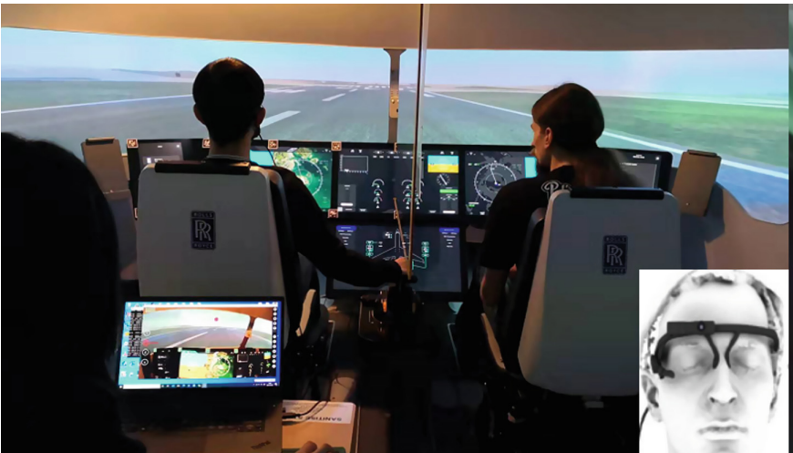
Fig. 2. Participant wears eye tracker performing landing scenario as pilot-flying interacting with touchscreen on Future Systems Simulator
