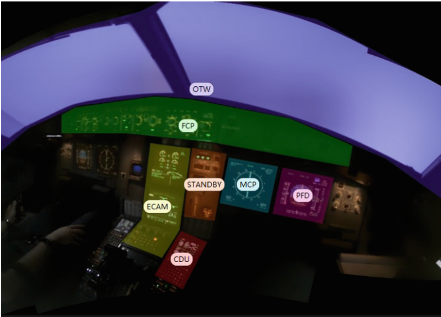
Fig. 2. Division of AoIs. Each color block represents a certain area of interest. The corresponding label on the color block suggests the name and function of the area. The remaining area that is not marked is seen as a whole.
