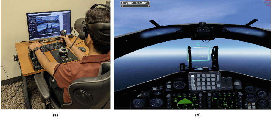
Fig. 1. (a) A user flying the Boeing T-45C jet using a HOTAS, and (b) a screen capture of the testbed in Prepar3D.
