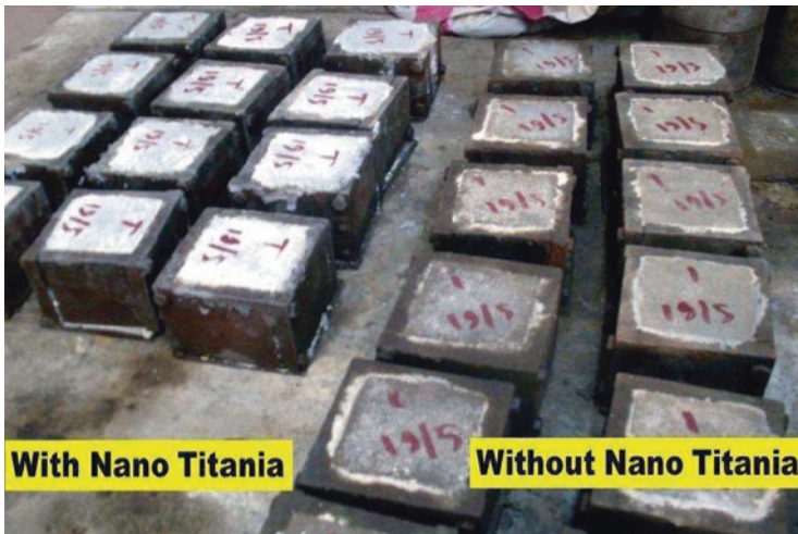
Fig. 11.5 Casted Nano Titania (NT) Cementitious Composites (left) and Reference Specimen (right)
