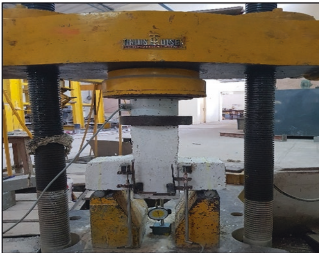
Fig. 10.3 Test set-up for column with double corbel
