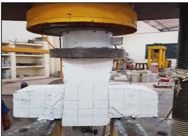
Fig. 10.5 Failure pattern for corbel with shear reinforcement
