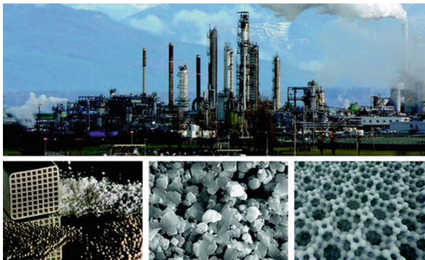
Fig. 10.1 Nanoporous materials (bottom right), available as crystallites (bottom middle), often in compressed form (bottom left), are key elements in refineries and other chemical plants for matter upgrading (top). The top picture was cut from an image by Walter Siegmund, licensed under CC BY 2.5 [5]. Bottom pictures reproduced with permission from Ref. [6], copyright (2013) Chemiewerk Bad Köstritz GmbH and Wiley-VCH Verlag GmbH & Co. KGaA
