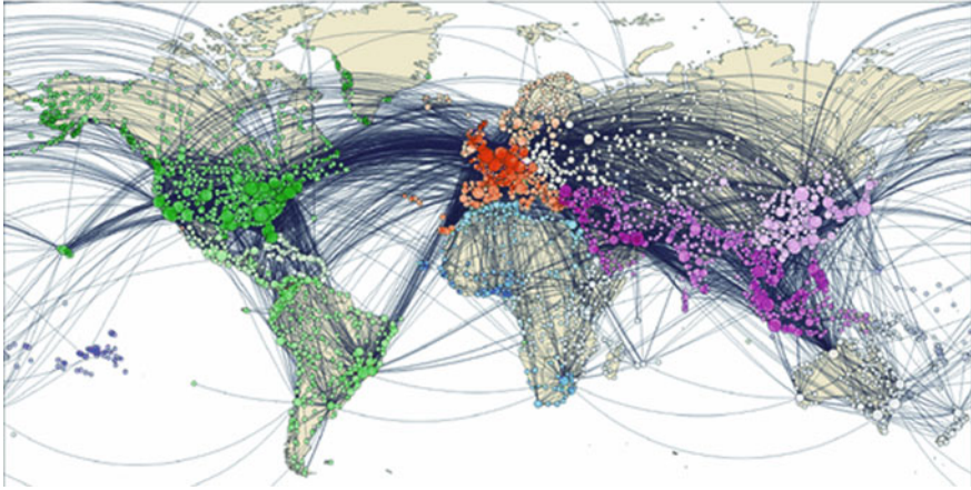
Fig. 20.1 The global air-transportation network. Each node represents one of approx. 4000 airports, each link one of approx. 50000 direct connections between airports. More than 3 billion passengers travel on this network each year. All in all every day more than 16 billion km are traversed on this network, three times the radius of our solar system
