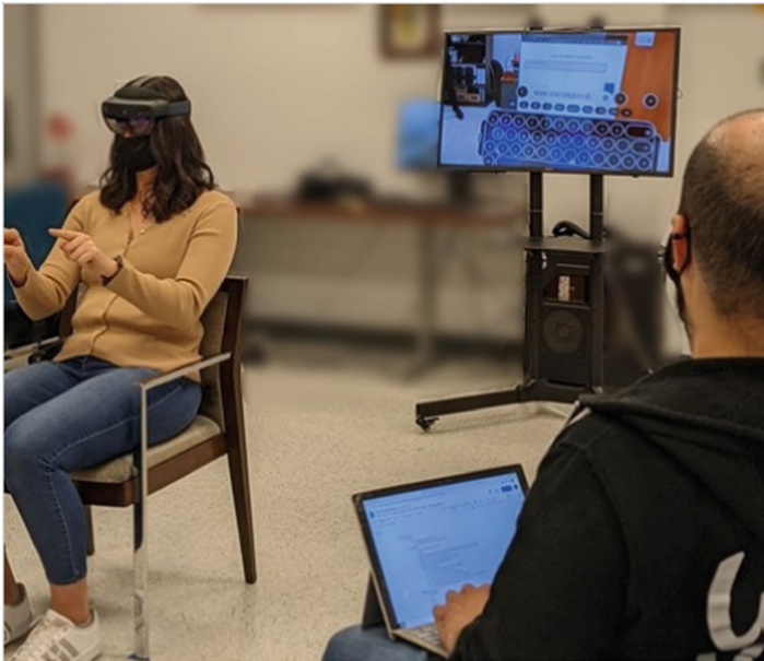
Fig. 2. Layout of experimental set-up, showing the participant completing the text entry task while wearing the HoloLens 2 (left) as the researcher (right) observes the participant's performance using the television screen and screen-mirroring device (top).
