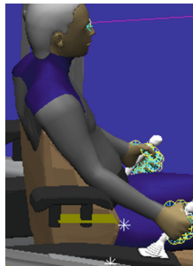
Fig. 13. Unrealistic manikin position using joint capacity analysis to modify the environment.
