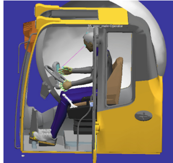
Fig. 10. Reach analysis of what environmental elements are within the manikin's reach.
