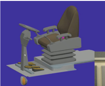
Fig. 4. (Left): The sitting section of the excavator. All other parts are being hidden.
