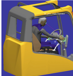
Fig. 9. Position of index and line of vision on the touchscreen.
