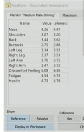
Fig. 24. (Right): the discomfort assessment of the second iteration
