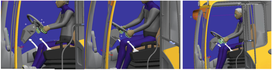
Fig. 7. From left to right, final steering wheel position for 5 th percentile female, 50 th percentile male, and 95 th percentile male.
