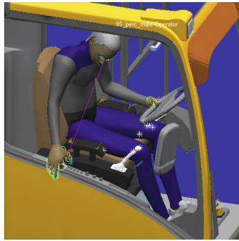
Fig. 11. Position of index and line of vision on actuating controls.
