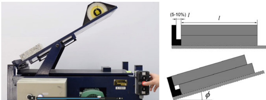
Fig. 10 Tilt test equipment (left), and schematic representation (right)
