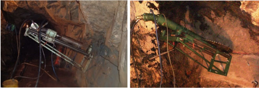
Fig. 20 Plate loading tests in an adit ( left ), and in a tunnel ( right ) [47]
