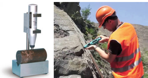
Fig. 13 Schmidt hammer and core holder (left), and used in the field (right)
