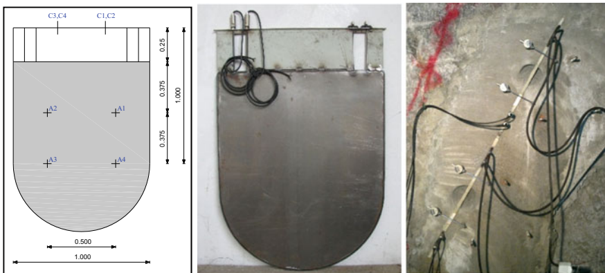
Fig. 21 Schematic representation of a large flat jack ( left ), a large flat jack ( centre ), and a LFJ test set-up with two jacks on a vertical wall of an adit ( right ) [47]
