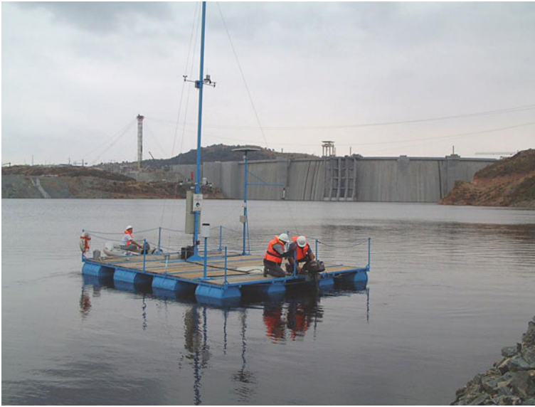
Fig. 2 Assembling and setting up a floating meteorological station, with underwater sensors for temperature and water quality implemented in the man-made lake of Alqueva in southern Portugal
