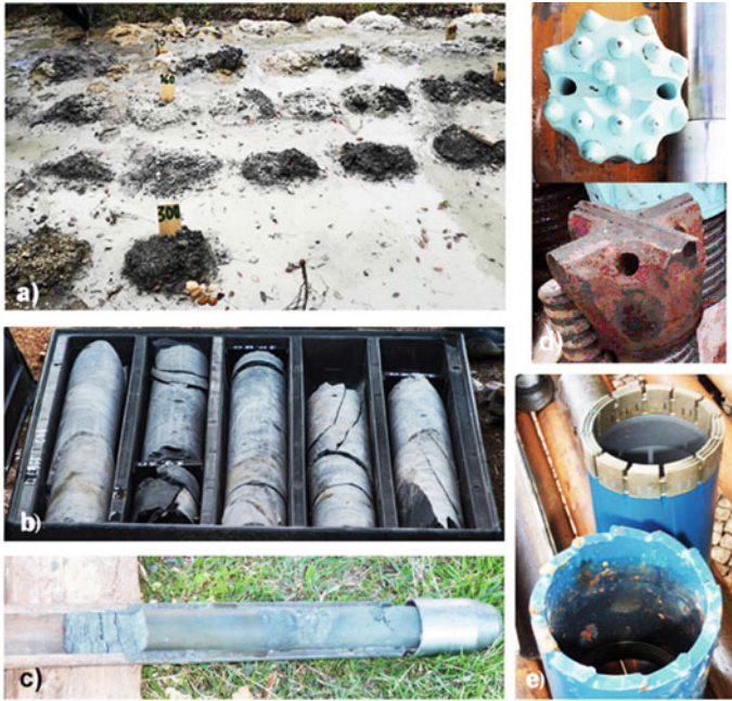
Fig. 6 Types of samples and core drilling bits: a cuttings obtained by destructive methods; b drill core; c opposing hemispheres of the split-spoon sampler open, exposing the recovered clay sample of an SPT test; d tungsten carbide bits for destructive drilling; e drilling bits for core sampling, diamond-impregnated and tungsten carbide tipped cutting shoe
