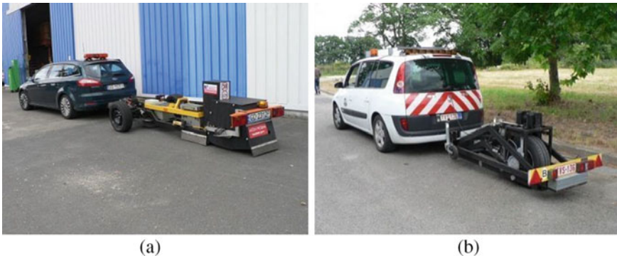
Fig. 12 Trailers for rolling resistance measurements, based on the angle measurement principle: a TU Gdansk trailer; b BRRC trailer. Photos by Anneleen Bergiers
