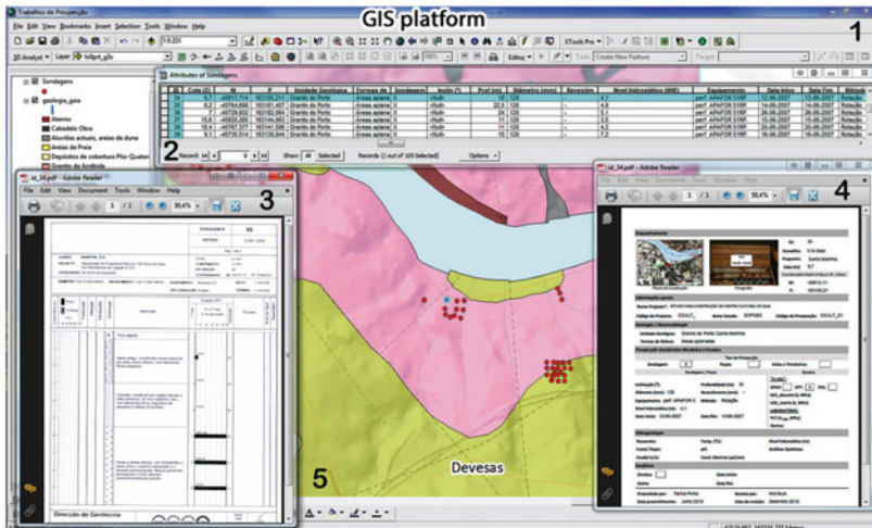
Fig. 5 Example of a conceptual flow-chart of the engineering geological map methodology for urban geoscience and municipal planning [30]: 1. GIS application tool creates hyperlinks between features (line, point or polygon) and other files; 2. Geo-database related to ground investigations information; 3. Geotechnical borehole datasheet; 4. Geotechnical inventory datasheet (field and desk data); 5. Detailed in situ investigation works mapping with geological background information
