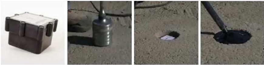
Fig. 4 Example of a vibration sensor [33]
