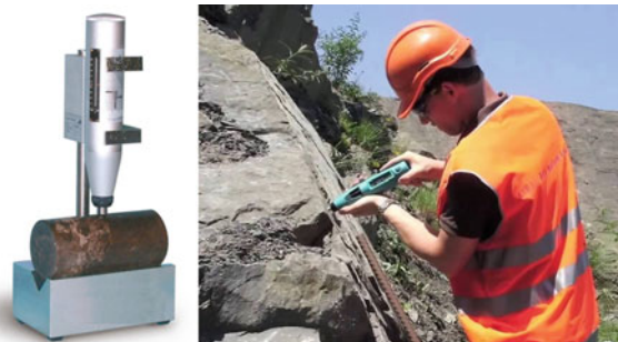
Fig. 13 Schmidt hammer and core holder (left), and used in the field (right)
