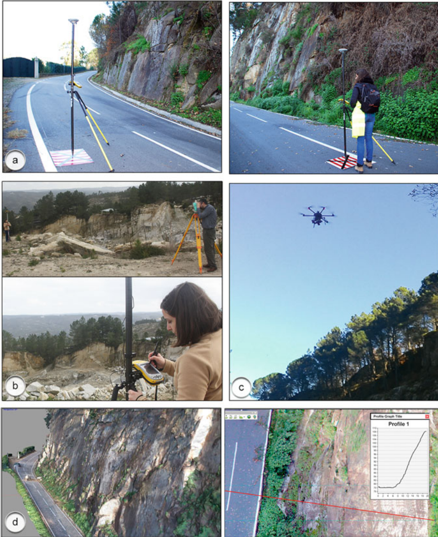
Fig. 3 Examples of geotechnologies used to support field mapping and in situ testing sites (images a) to (c) from LABCARGALISEP archive; (d) kindly shared by José Filinto Trigo, NECIISEP); a, b high-resolution global positioning system (GPS) in rock slope geotechnics studies and total station in surveying studies to support digital photogrammetry techniques ( b ); c unmanned aircraft vehicles (UAV) to support detailed mapping and terrain modelling with 3D rock slope model resulting from UAV aerial surveys ( d )
