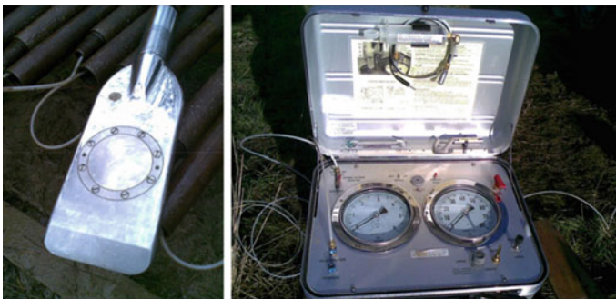
Fig. 8 Flat dilatometer and measuring equipment (courtesy of Geocontrol)
