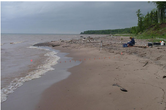
Fig. 4 Example of field measurements of wave run-up using markers (orange marks) and a video-camera mounted on a tripod (from Swenson [17])
