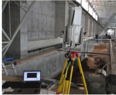
Fig. 17. 3D scanner used in dam-breaching tests
