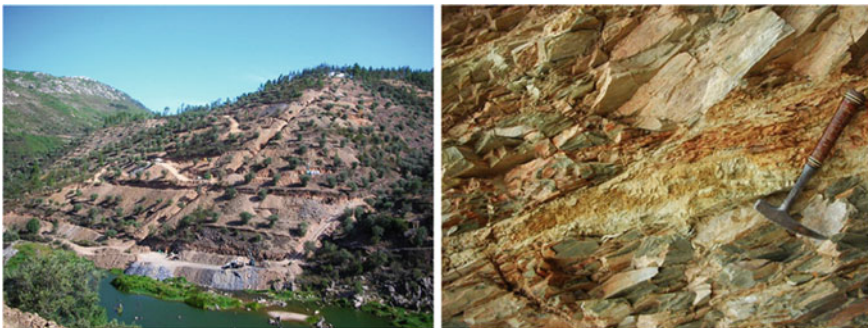
Fig. 5 Trenches excavated to investigate a dam site (Portugal) ( left ) and a detail of a fault containing clay gauge observed in a trench wall ( right )
