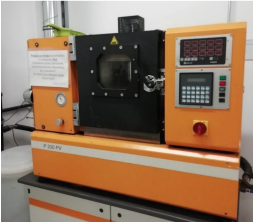
Fig. 7.8 Vacuum press for sample preparation for rotational rheometry and thermal conductivity (Source MUL facilities)
