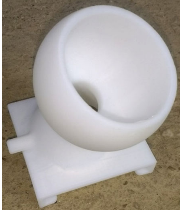
Fig. 2.15 Finished ABS part manufactured on an FFF machine (Photo by Tomislav Breški)
