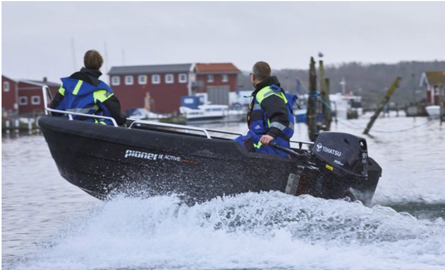
Fig. 6.92 3D printed boat from RISE and Cipax (Courtesy of RISE, Photographer Anna Hult AB)
