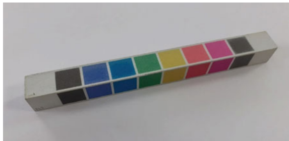
Fig. 2.8. 3D-printed part with variable colour (Photo by Tomislav Breški)
