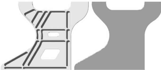
Fig. 5.2 Left: Original part intended for manufacture. Right: Simplified model intended for optimization (Courtesy of Axel Nordin, original model by Olaf Diegel)
