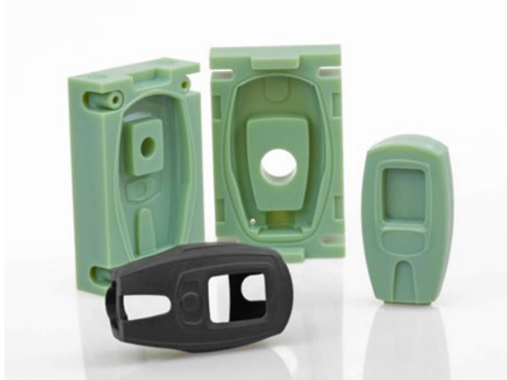
Fig. 1.11 Injection mould made by PolyJet Matrix (Courtesy of Stratasys )
