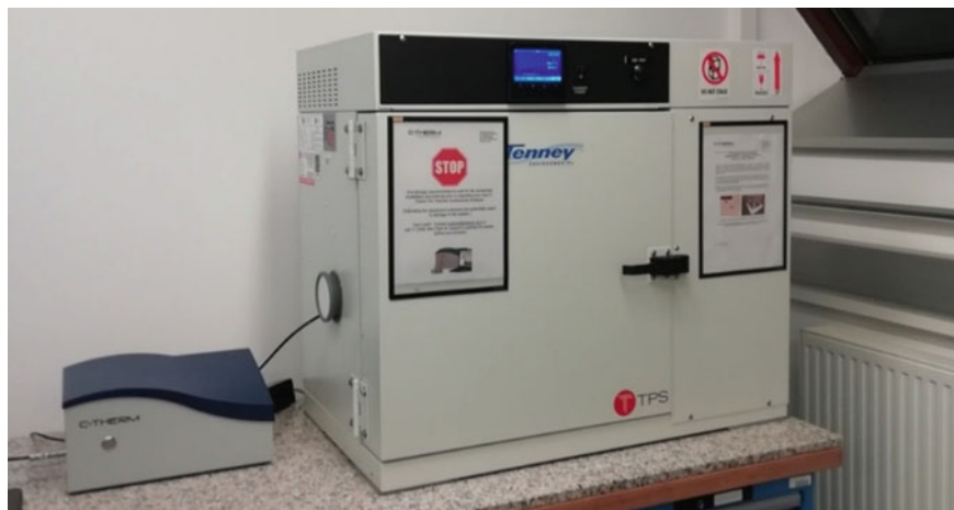
Fig. 7.10 Thermal conductivity device that uses the modified transient plane source method (Source MUL facilities)
