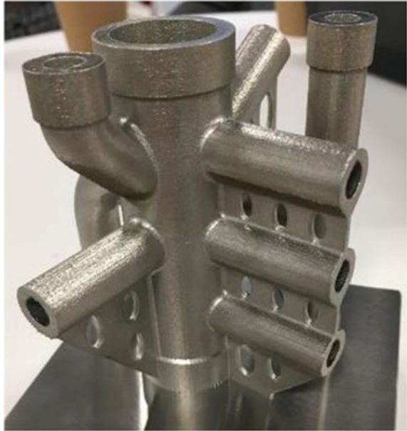
Fig. 4.9 A designed for AM block manifold with reduced print time and support removal time (Courtesy of Olaf Diegel [1])
