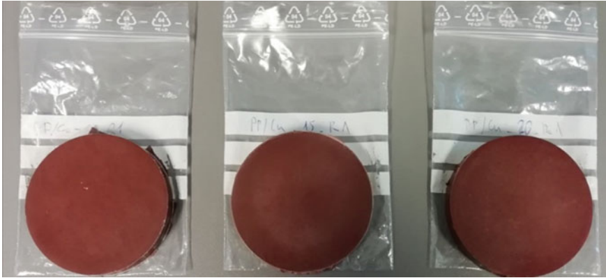
Fig. 7.11 Samples for thermal conductivity measurements prepared in the vacuum press ( Source MUL facilities)
