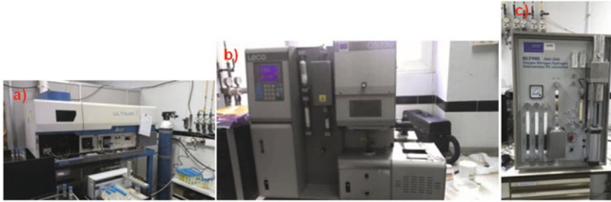
Fig. 7.22 Equipment for chemical analysis characterisation at AIDIMME: a Ultima2 (ICP-OES), b Leco CS230 and c ONH-2000(IGF) ( Source AIDIMME facilities)
