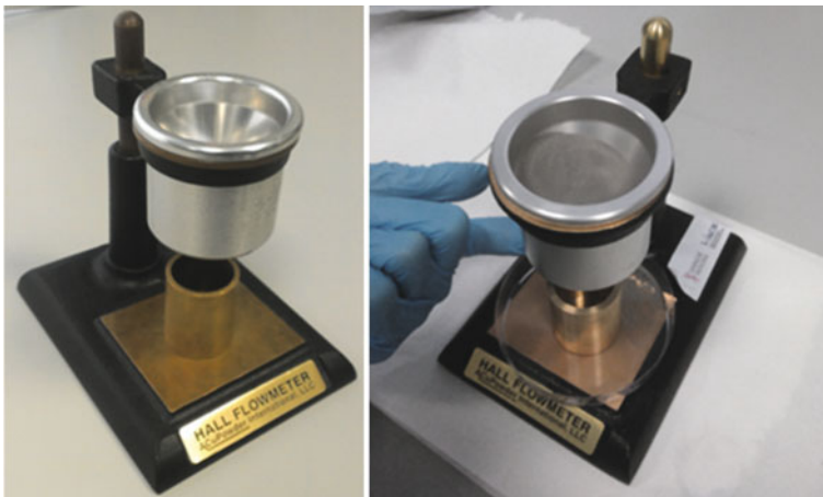
Fig. 7.24 Hall flow rate equipment (Source AIDIMME)
