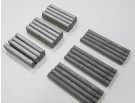
Fig. 7.36 Tensile bars together with samples for microstructure and porosity testing ( Source RepAir project, AIDIMME)
