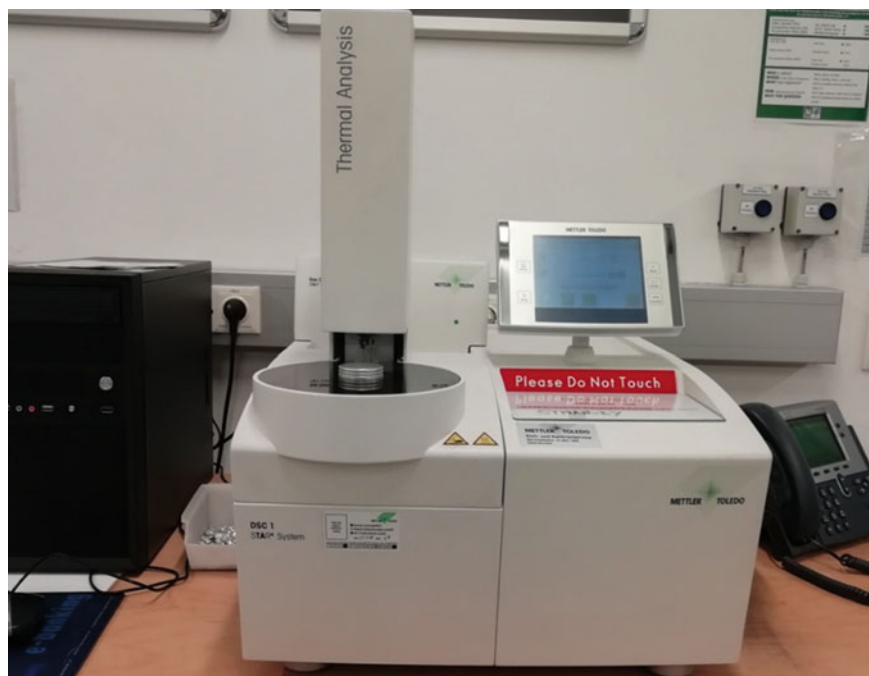
Fig. 7.6 Differential scanning calorimetry device ( Source MUL facilities)
