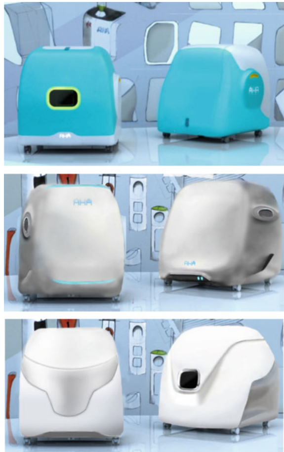
Fig. 2 Different design concepts worked out in the user-centered design sessions that illustrate the shape and color of the PEPE mobile platform when parked. The size is approximately of 80 \times 60 \times 60 cm. All designs consist of a wheeled platform that contains all hardware components, with openings for the floor projection and depth sensor, and a lid on top to uncover the access to the monitor and computer system
