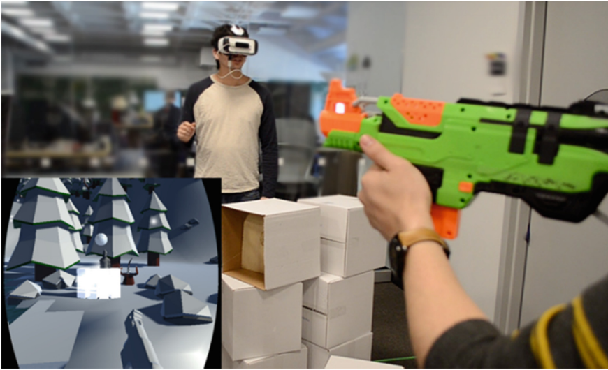
Fig. 7 SnowballVR showing two users, one shooting virtual snowballs using a modified Nerf gun and the other dodging the snowballs by hiding behind a physical/virtual snow fort. Figure from the paper (Sra et al. 2016)
