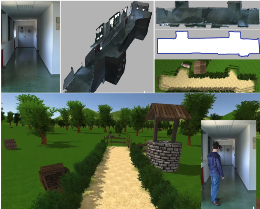
Fig. 3 Oasis system creates a 3D map of the physical environment, automatically detecting open walkable areas which allow the system to generate virtual environments with corresponding walkable areas. While the physical affordance of walking is the same in both environments, the visual experience and spatial feel can be quite different. For example, as seen in the figure above, a hallway is transformed into an open countryside which still allows the user to walk freely while wearing a wireless headset device in the mapped physical/virtual space without breaking immersion. Figure from the paper (Sra et al. 2016)
