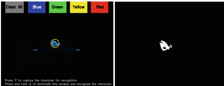
Fig. 5. Left: Tracker detection feedback in the live viewer with ROG phone's RGB logo as the tracker. Right: Mask formation of the detected tracker with suppressed noise.
