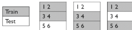
Fig. 2. Total 6 data sample is used. Highlighted boxes show training data and other are testing dataset. As k’s value is 3, total three folds created with 2 datasets where each sample goes for training and testing during any of the fold execution.
