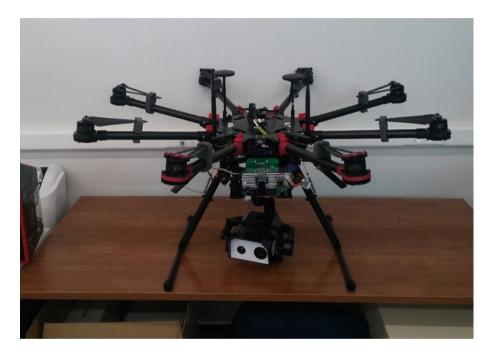
Fig. 2. The octacopter UAV
