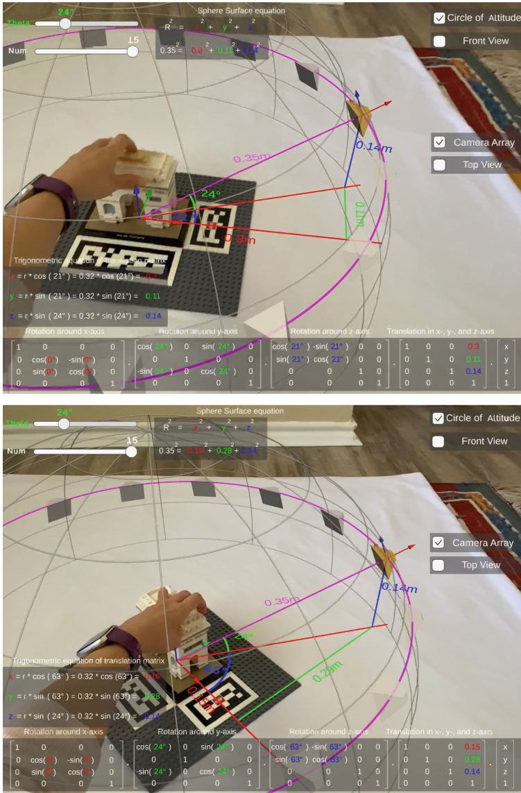
Fig. 7. While student transforms the physical LEGO model from pre-image on the top to image on bottom, the spatial graphics and math representations update in real time accordingly.
