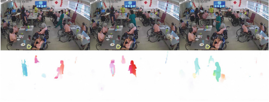
Fig. 6. Staff movement in the patch using optical flow estimator
