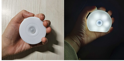
Fig. 12. Making prototypes to offer a dim light when detecting movement in a dark environment
