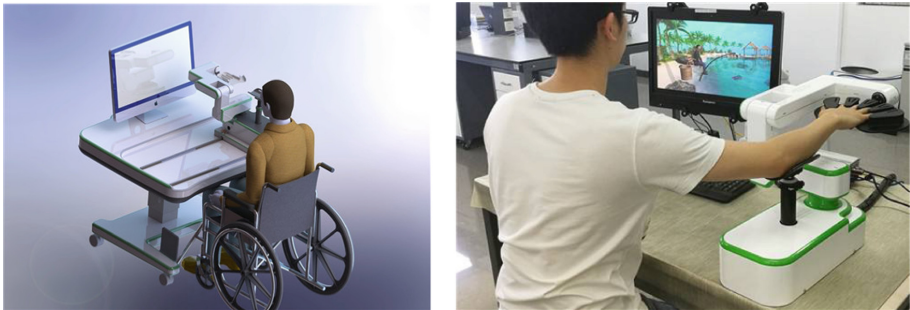
Fig. 1. A prototype of three degrees of freedom wrist motor function rehabilitation training system based on scenario interaction.
