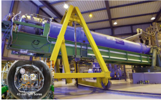
Fig. 3 The CAST experiment with a close up photo of the twin bores where CAST-RADES and CAST-CAPP microwave cavities are installed (CAST credits)
