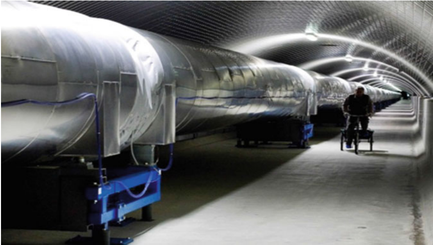
Fig. 5 The 3 km vacuum tube inside the Virgo North galler (Credits The Virgo Collaboration)
