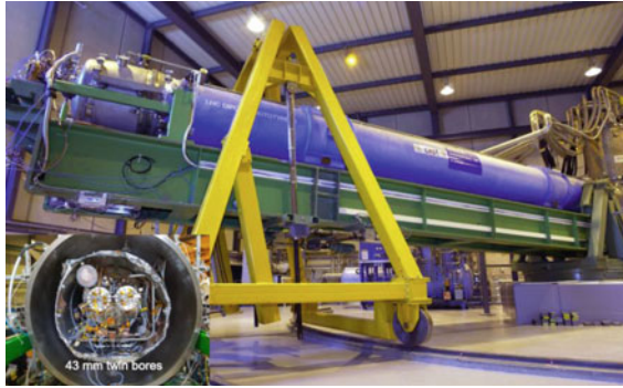
Fig. 3 The CAST experiment with a close up photo of the twin bores where CAST-RADES and CAST-CAPP microwave cavities are installed (CAST credits)
