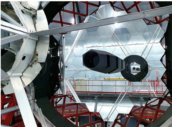
Fig. 7 The segmented primary mirror of the 10.4 m GTC telescope, at present the largest optical-infrared telescope in operation. Note the different reflectivity of the segments due to oxidation, each segment is re-coated once a year (credit G. Gomez Velarde)
