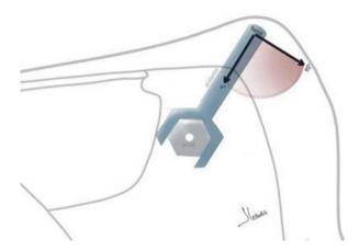
**Fig. 10.20** The moment of a force. The moment of force depends on the distance and force applied. It represents the capacity to rotate an object around a pivotal point. If the force is perpendicular to the distance  $(90^\circ)$ , we achieve maximum rotation. If the force is performed in the same vector of distance  $(0^\circ)$ , the moment of the force is 0, and there is no movement. It is fundamental to choose the ANSA banner angle that must follow the LC long axis vector
