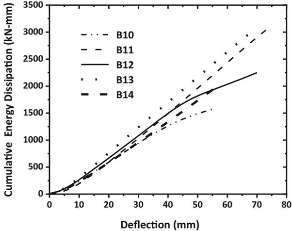
Fig. 3. Cumulative energy dissipation vs deflection.
