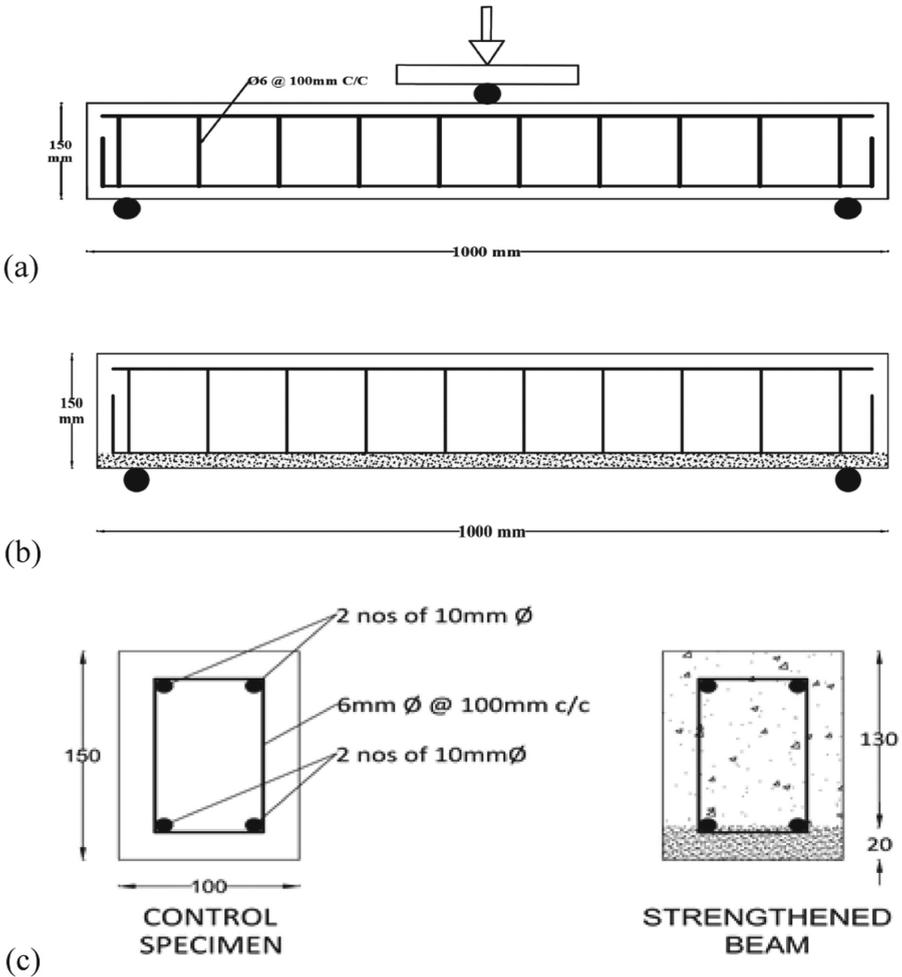
Fig. 1. Beam specifications-(a) Control specimen; (b) Strengthened beam; (c) Sectional view.
