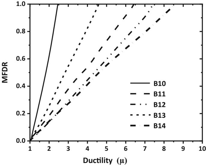
Fig. 5. Modified flexural damage ratio.
