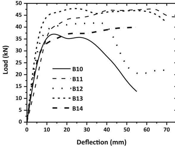
Fig. 2. Load vs deflection behavior of RC beams.
