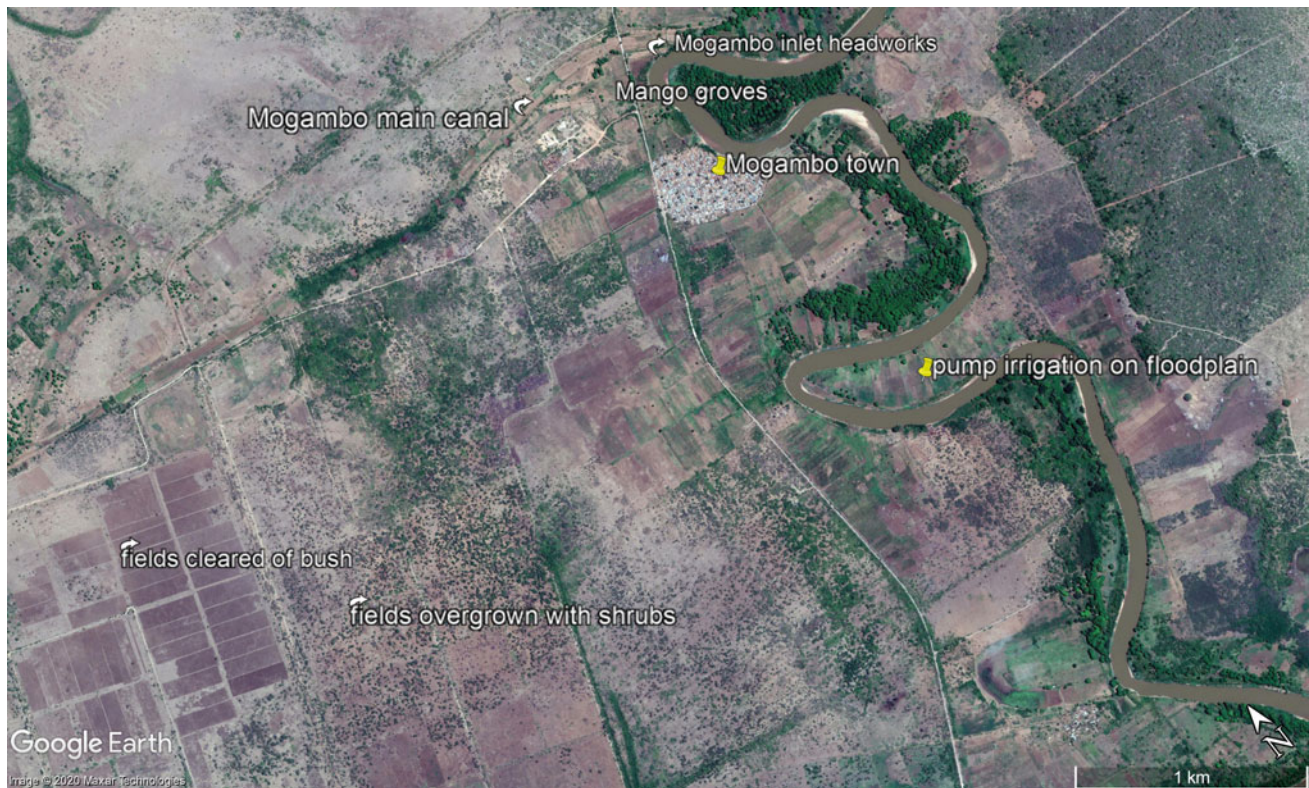
Fig. 14.24 Enlargement of the MIP scheme in January 2016 showing inactive state. North at top. Google Earth ©
