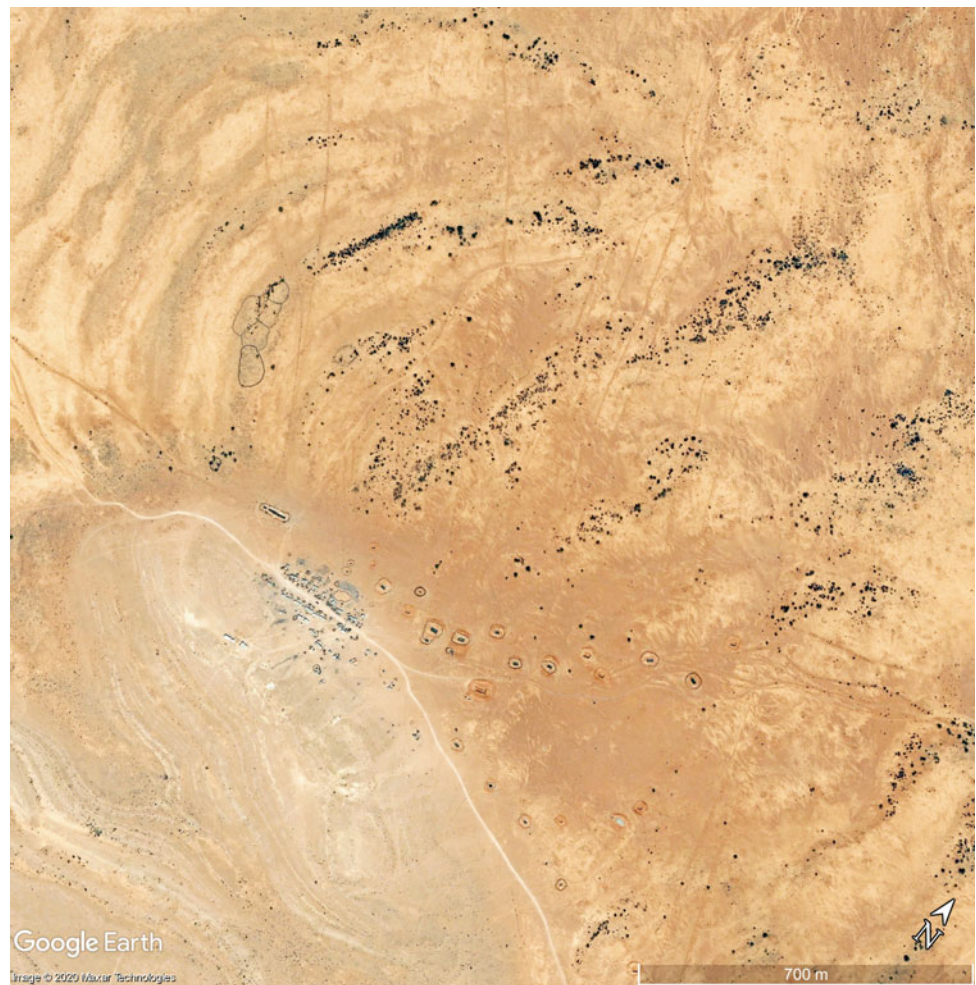
Fig. 14.49 Enlargement of a set of arcs from Fig. 14.48b. The settlement (at 9^{\circ}38'46.18''\text{N} , 49^{\circ}34'15.52''\text{E} ) is near the Bur Aden hills, some 56 km NE of Qardho. A pastoral area too dry for rainfed farming, tanks have been dug in the bedrock to harvest run-off. Woody vegetation occupies some of the arcs showing the stable nature of the arc, but some have lost their vegetation. Google Earth © 2004 imagery
