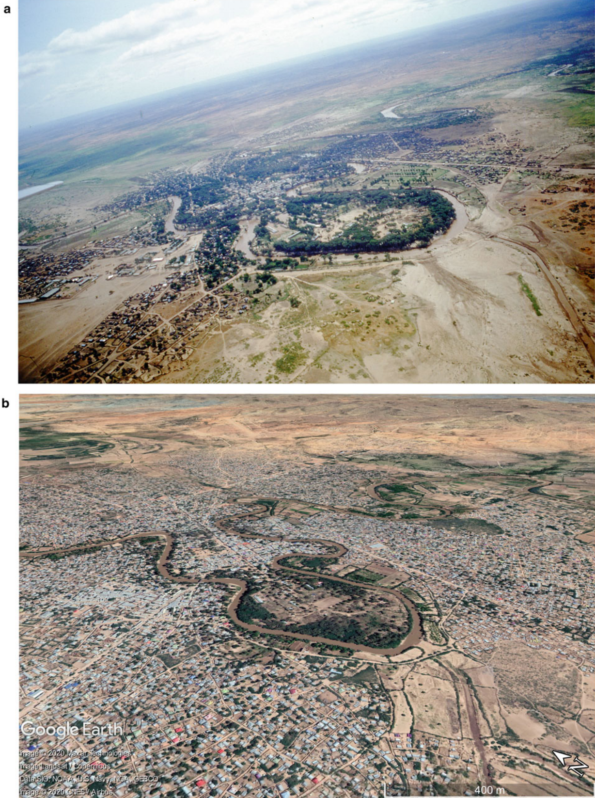
Fig. 14.14 a Beled Weyn crevasse splay and flooding in the town, bypassing the flood-relief channel. Downstream is to right. Photo RN Munro ©, 28 June 1981. b Approximate same view generated from Google Earth ©. The town has expanded; the flood-relief channel had
