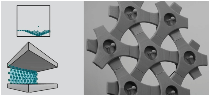
Fig. 8. Right: digital model of the reTessellate. Left: assembled physical model using a triangular repetitive structure and linear actuator modules.
