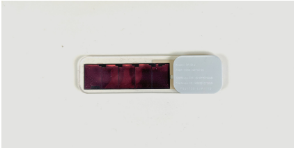
Fig. 2. Solar-powered BLE beacon (PulsarGum TM-010 made by Fujitsu).
