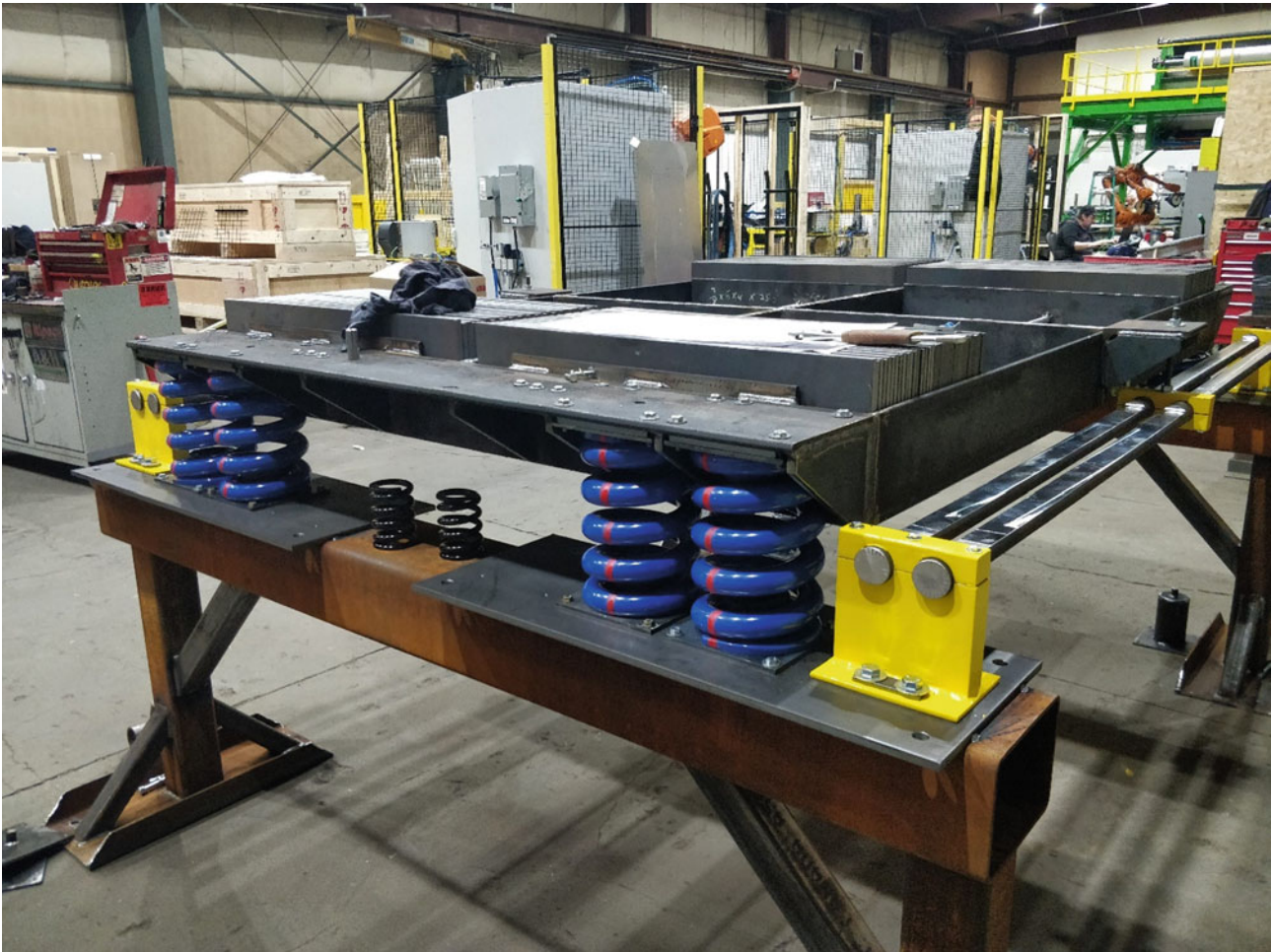
Fig. 2.2 TMD test frame for shop testing
