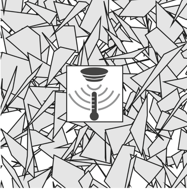
Fig. 4. AR marker of the microcontroller system with the SHT-31 sensor. The symbol in the center of the AR marker is used for identification by the user.
