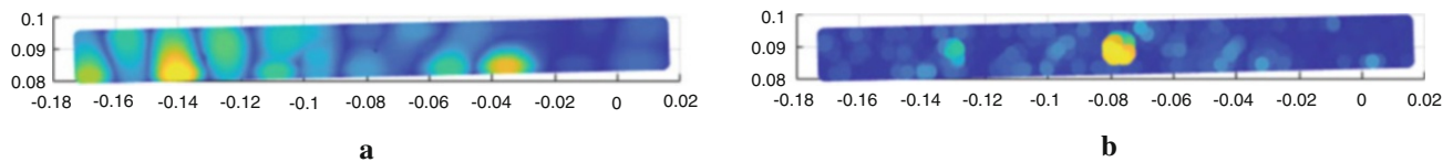
Fig. 14.9 Absolute magnitude of (a) high-frequency mode shape and (b) the corresponding second derivative
