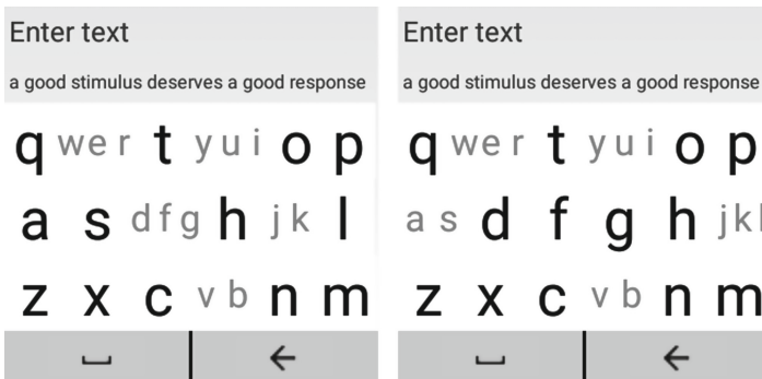
Fig. 1. BubbleBoard static layout (left) and example expansion of the f character (right).
