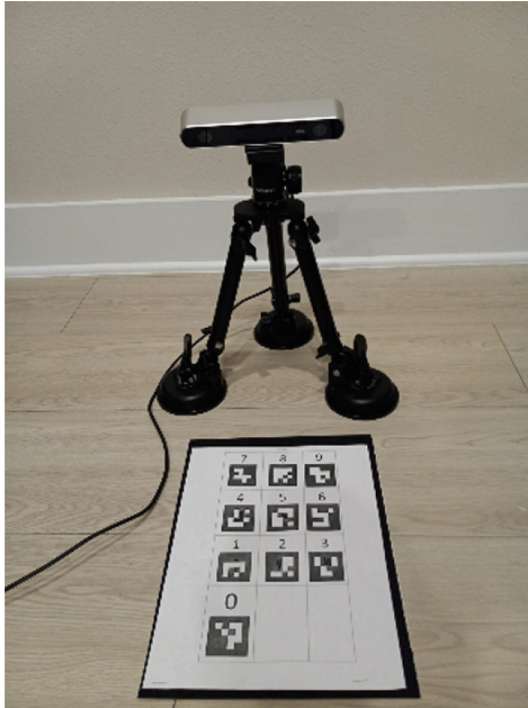
Fig. 2. Stereo camera (USB3 ZED camera) based ArUco keyboard system.
