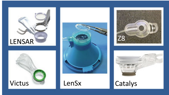
Fig. 6 Patient interfaces for the laser systems listed in Table 1. The LenSx interface uses soft and flexible hydrogel inserts, which need to be assembled and matched to the patient’s corneal curvatures. All others utilize water immersion with a scleral suction ring
