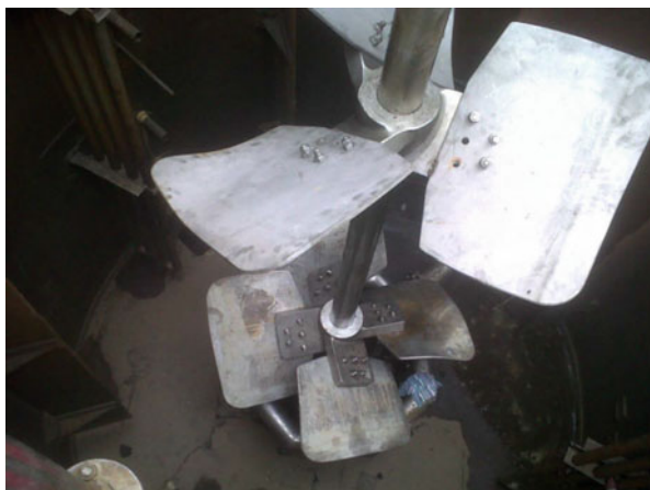
Fig. 12.3 The dual P4/P3 impeller system in the three primary bioleach reactors at the Mondo Minerals nickel sulfide plant
