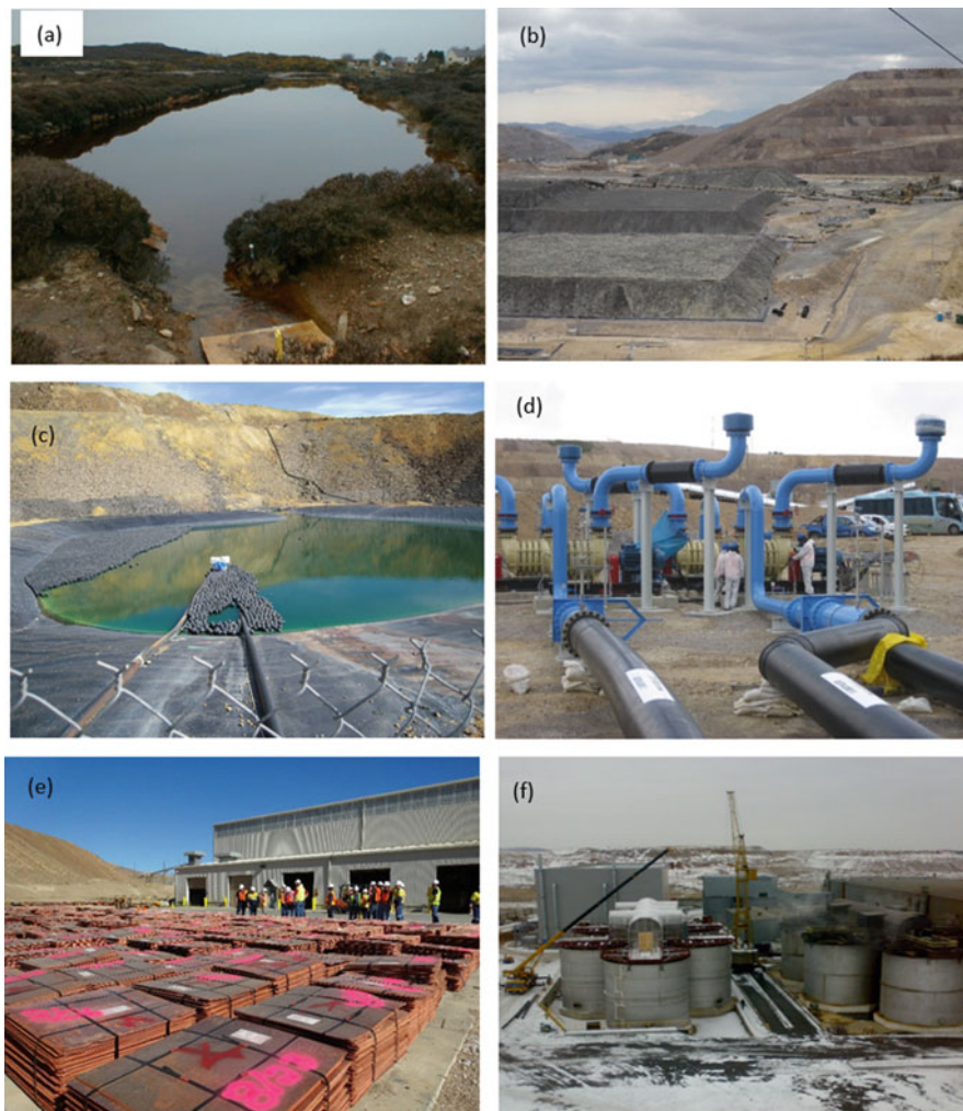
Fig. 1.1 Images from sites where different approaches are used to bioleach or biooxidise sulfidic ores and concentrates to recover base and precious metals. (a) precipitation pond, used to recover copper from in situ bioleaching (Mynydd Parys, Wales); (b) run-of-mine and crushed ore bioleach heaps (Yanacocha mine, Peru); (c) pond receiving copper-rich pregnant leach solution from a trial heap leach (Bingham Canyon mine, Utah); (d) bioleach aeration blowers and distribution plenum (Yanacocha mine, Peru); (e) copper cathode produced by SX-EW (Phoenix mine, Nevada); and (f) continuous stirred tanks used to process refractory gold ore (Suzdal mine, Kazakhstan)
