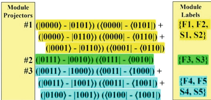
Fig. 7.13 Command Design Pattern modules—Obtained by partitioning projectors into three disjoint sets (in different colors), in the figure middle. Structors and Functionals are seen in the figure r.h.s.
