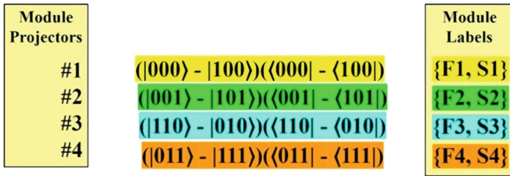
Fig. 7.6 Deutsch algorithm modules from projectors—There are four modules, obtained from the density matrix in Fig. 7.5. The scaling factor was omitted for clarity in each module
