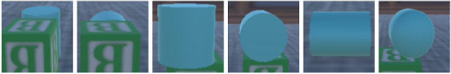
Fig. 10. Sample of misrecognized objects. From left: cylinder misrecognized as cube (1), and capsule (2), cylinder misrecognized as cube (3), sphere (4), and capsule (5), and capsule misrecognized as sphere (6).
