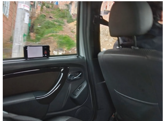
Fig. 2.9 Side mounting of cell phone enables mobile street view image collection
