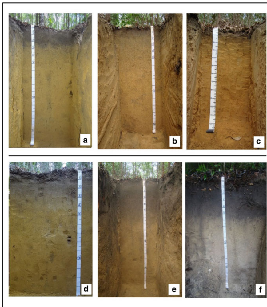
Fig. 6 Latossolos Amarelos Distrocoesos (Xanthic Ferralsols) profiles present in the Dissected tableland (a–c) and Tablelands (d–f) compartments
