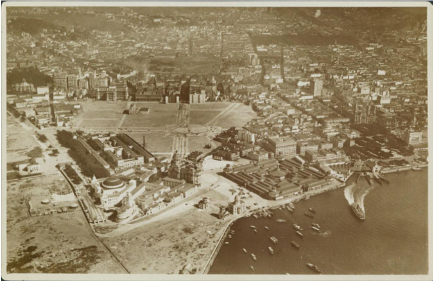
Fig. 10 Photograph of the esplanade of Castelo hill in 1930, a few years after its dismantlement, where the immense urban void stands out amidst the nineteenth- and early twentieth-century houses. This esplanade is positioned 5–8 m above the base level of the surrounding plains. It can be seen, on the left, an extensive area that has just been reclaimed along the Guanabara Bay. Source Holland (1930?)
